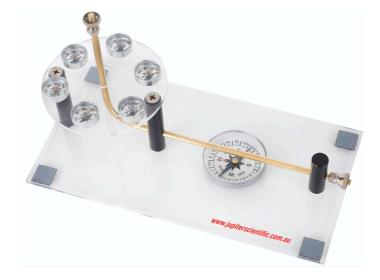
The *Ampere Rule* may be used to demonstrate this concept. The apparatus consists of a thick 'L' shaped wire mounted on a clear acrylic base, a number of small compasses, and a large compass.
